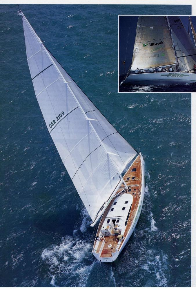
Pinta Smeralda has topped 15 knots downwind and makes a good 9 upwind. Her big rig on a carbon spar is nevertheless simplicity itself to control, the mainsail slipping so unobtrusively into the boom and the slightly overlapping headsail furled at the press of a button by the helmsman from his steering console
